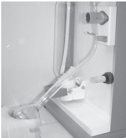
Placement for the collector flask to add drops to near the graduated mark.
