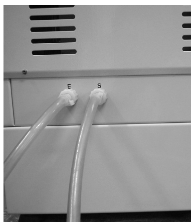
Fig 4.3: Inlet and outlet water connections
