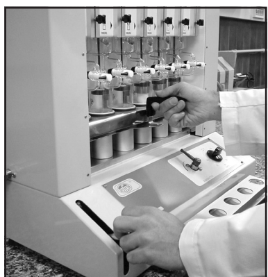
Placing the beakers on the extraction unit
