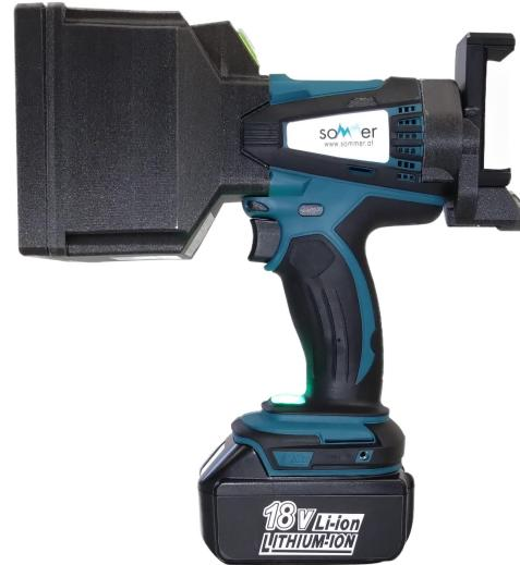
The HSR-10 mobile handheld radar sensor is a measurement device for the contact-free determination of the flow velocity of open rivers and channels. The sensor detects the surface flow velocity by the principle of the Doppler frequency shift.
