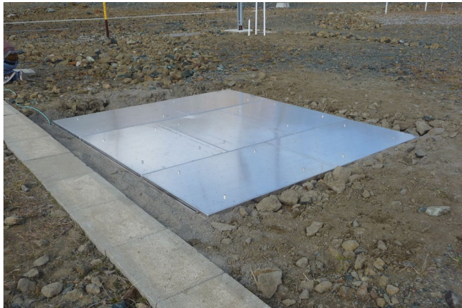
Figure 4: 已安装的SSG 雪量计
